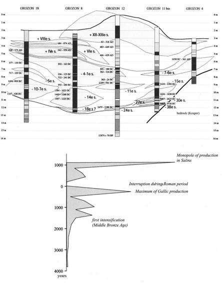
Figure 4. Salt exploitation in Grozon (Jura, France): Longitudinal stratigraphic cut of the Grozon basin (400 m) based on drill cores and dated by radiocarbon. The depression was created after the underlying salt-rock was dissolved (top). Schematic chronological evolution of the charcoal sediments volume related to salt exploitation (bottom) (drawings P. Pétrequin).
