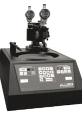
The MultiPrep™ System enables precise semiautomatic sample preparation of a wide range of materials for microscopic (optical, SEM, FIB, TEM, AFM, etc.) evaluation. Capabilities include parallel polishing, angle polishing, site-specific polishing or any combination thereof. It provides reproducible sample results by eliminating inconsistencies between users, regardless of their skill.
